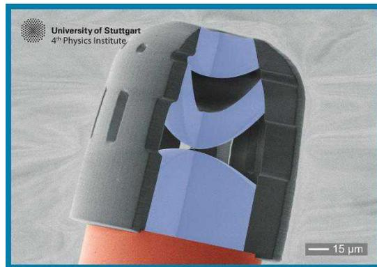
Atomic layer deposition yields antireflection coatings on all optical elements. Confocal surface profiling and wavefront interferometry demonstrate accuracies far better than  $\lambda/20$ . In combination with high-resolution nanostructuring, also 3D holograms and metasurfaces can be included.
